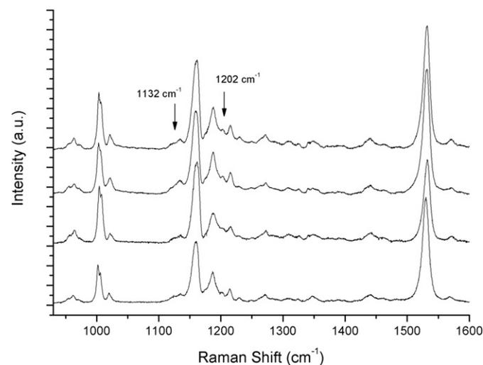
**Fig. 4.** Resonance Raman spectra (488.0 nm excitation, leading essentially to neoxanthin contributions) of (from bottom to top) purified LHCII from spinach, LHCII reconstituted from WT Lhcb1 apoprotein from pea, LHCII reconstituted from S123P Lhcb1 apoprotein, and LHCII reconstituted with S123G Lhcb1 apoprotein. Spectral range displayed: 930–1600  $\text{cm}^{-1}$ .
